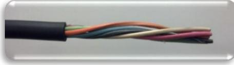
Remove about 3" of insulator from Cable.
