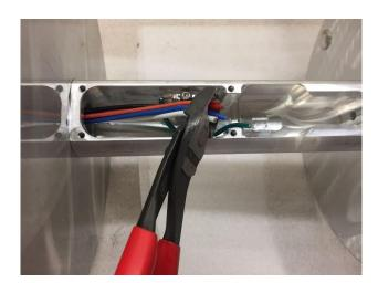
Feed the remote cable you've prepared through the connector on the Junction box cover, (Cover is in a bag in the box, along with 4 screws) slide it back on the wire, out of your way.
