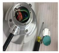
Using the # 8 screwdriver remove the ground screw separating the two ground wires, next use the needle nose pliers, reach inside the junction box Gently draw all the wires out of the box, disconnect the wires by removing the wire connectors, then separate the wires.
