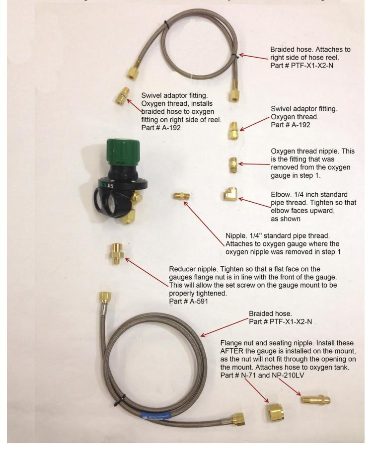
Step 3: Assemble acetelene gauge and parts as shown. Use teflon on threads with no seating end. Read all instructions before you start. Do not overtighten.
