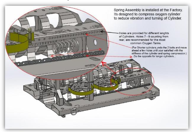
**Step 11:** Identify and install the oxygen tank holders. The removable half moon on the holder should be facing down. Right and left tank holders are provided.
