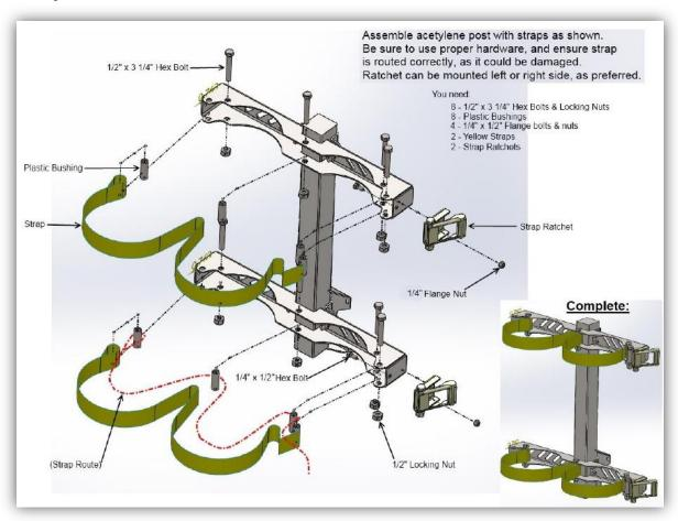
**Step 7:** Secure acetylene tank post to skid base.
