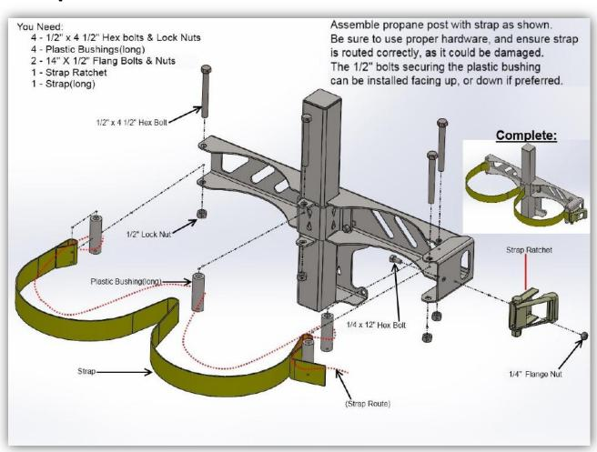
**Step 9:** Secure propane tank/ reel post to skid base
